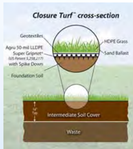
Sand is applied as a ballast eliminating the need for anchoring.
